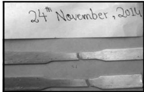
Figure4. Necked gauge width of fractured tensile test specimen
