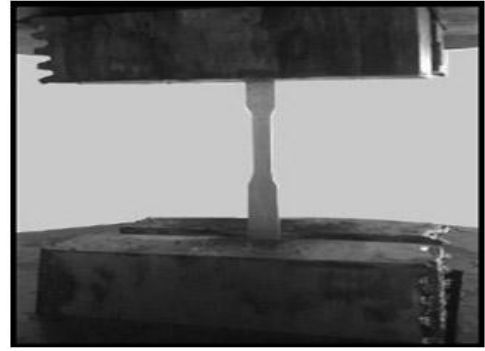
Figure3. Tensile testing specimen within the jaws of crosshead
